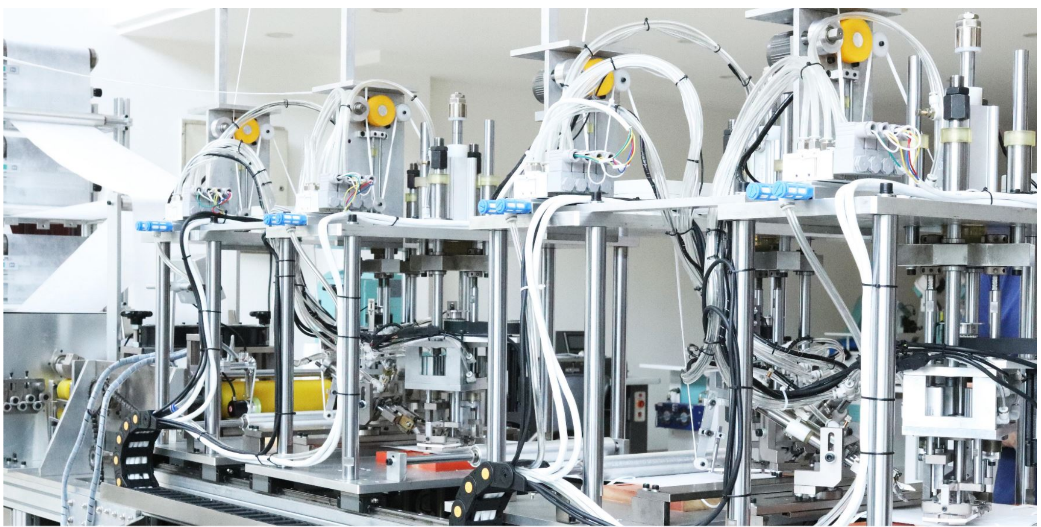
耳带点焊 Ear Loop Welding Unit
