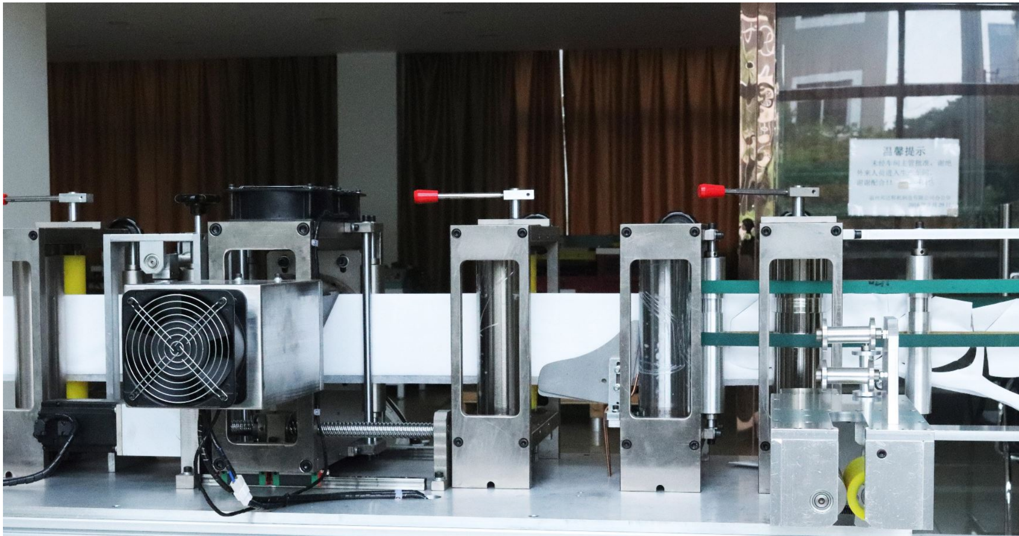
口罩封边、剪切 Face Mask Body Side Welding & Cutting
